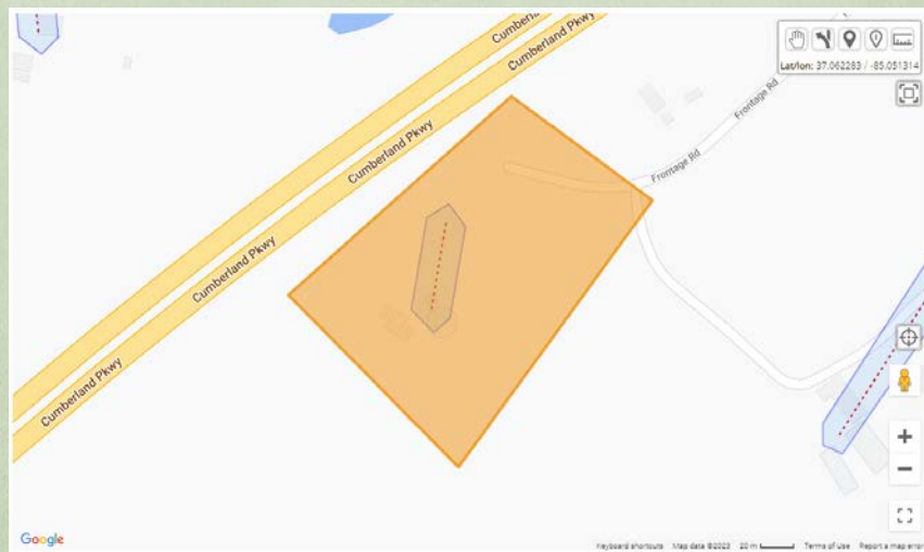
This shows the dig site location (orange polygon), the utility's notification area (blue polygon) and the facility centerline (red dash line - provided via WMS links for display)
