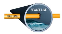
causing the blockage. If this is the case, the mechanical rotary device may cut through the natural gas line releasing flammable and dangerous gases into your home. This may result in a significant accident that could cause damage to property, cause injury or even death.
