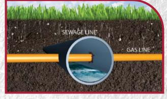
tool can damage a natural gas line that has been unknowingly bored through a sewer line. Natural gas can then migrate through the sewer line into a connected structure, including one without natural gas service. This migration creates the potential for a natural gas accumulation and possible deadly ignition.
